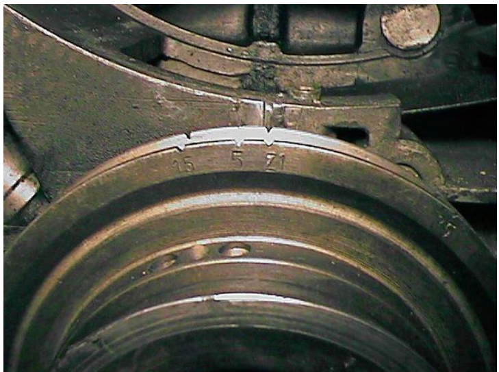
Figure 12: TDC 'Z1' Mark Aligned with Case Centerline
